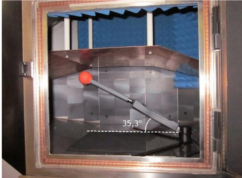
Figure 1: Calibration set-up in the absorber loaded TEM cell
